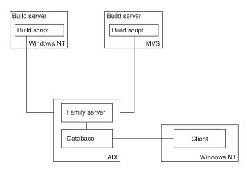
Figure 47. TeamConnection components on separate machines
